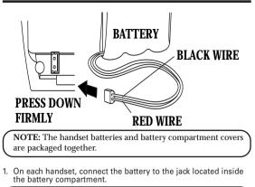
**NOTE:** It is important to maintain the polarity (black and red wires) to the jack inside the compartment as shown in the illustration
